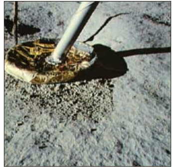
A foot-pad of Apollo 14, showing the surface texture ranging from dust to small rocks. Apollo 14 landed in the lunar highlands near the crater Fra Mauro.
